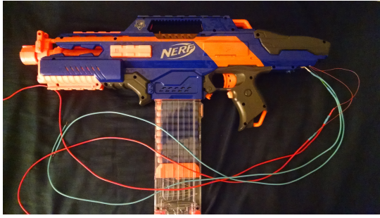
Fig. 3. The CS-18 that has been modified to allow external control.
