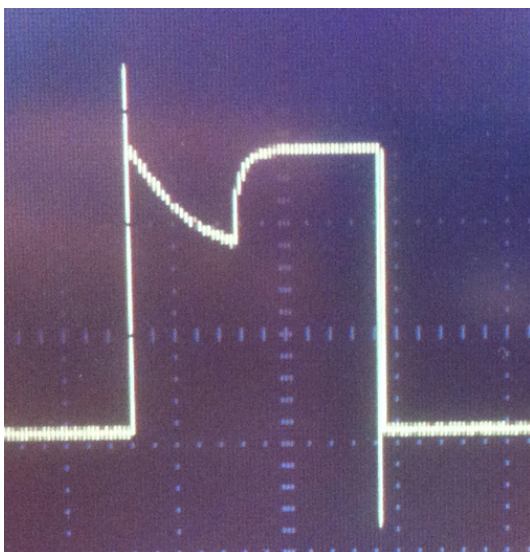
Figure 8: Faulty PWM Signal
