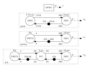
Figure 1: Successive refinements of an MP3 play-back application.
