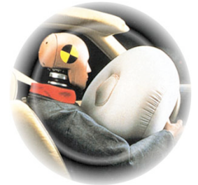
Side airbag in car, Reaction in <10 mSec
