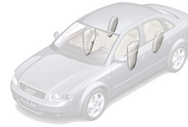
Side airbag in car, Reaction in <10 mSec
