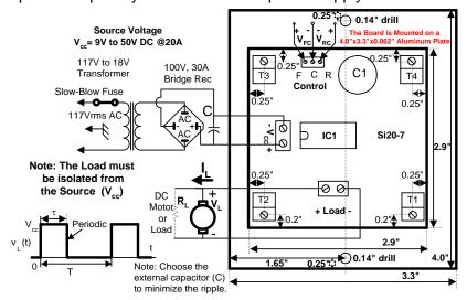
Warning: The connecting wires to the Load and the Power Supply must be heavy gauge copper wire (#12 AWG or heavier) to handle the rated current level. In addition, these heavy gauge wires act as a heat sink, protecting the board from overheating.
