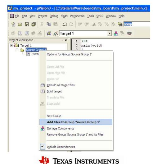
This process gives you the most basic project that will run on a Stellaris microcontroller. The next steps include configuring your project for your specific board, adding the hooks for StellarisWare, and setting up the debug and flash programming environment.
