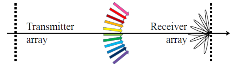
Data streams mapped onto angles of arrivals for linear arrays
