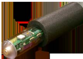
MIR integrated with Mica-2 Packaging to allow antennas to land pointing up
