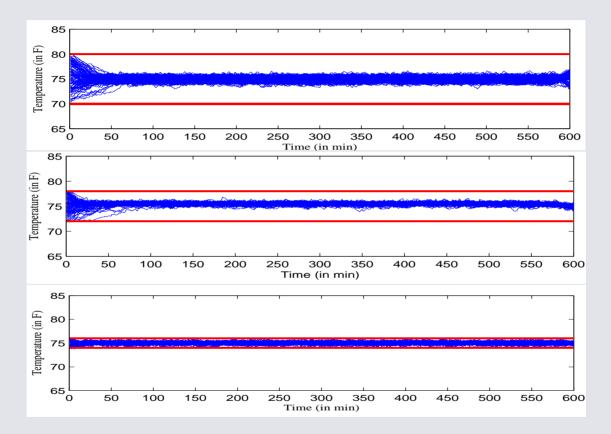
• Executions generated by optimal policy for three safe sets:  $(70, 80)^{\circ}F$ ,  $(72, 78)^{\circ}F$  and  $(74, 76)^{\circ}F$
