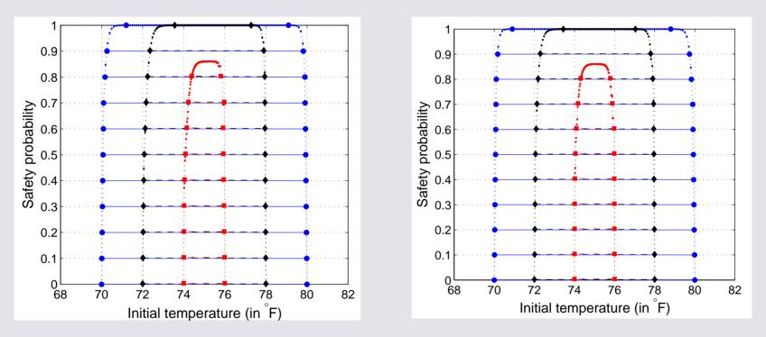
Maximal probabilistic safe sets for the three sets for different safety levels when the initial mode of heater is "OFF" and "ON" respectively
