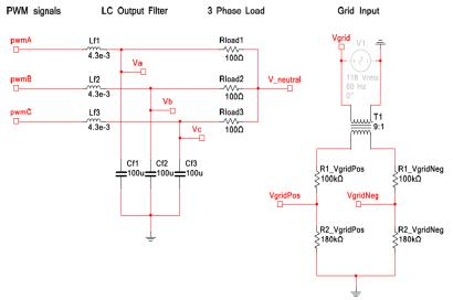
Fig. 2: Circuit schematic for the 3-phase output filter and load (left side) and the circuit used to convert the grid voltage levels to voltage levels within the range supported by the FPGA.
