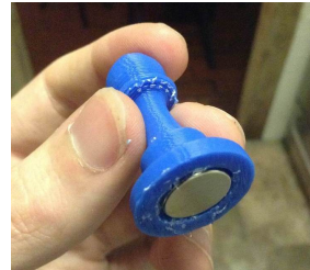
Each of the chess pieces are 3d-printed such that magnets can be placed in each one.
