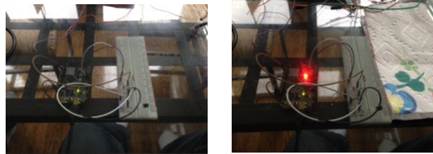
Figure 5 - Hardware Prototype displaying IR sensors working through glass table
