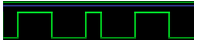
Fig. 7. Wave form of 0x93 (0 1100 1001 1) including framing bits, in the order of LSB
