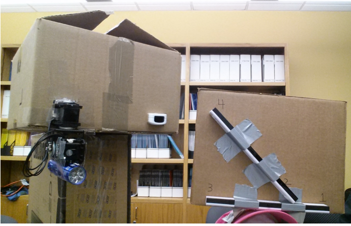
Fig. 2: SHAZam External Hardware. On the left, the main console with a protruding Wiimote camera and a Dynamixel 2-axis motor assembly with an attached flashlight. On the right, the head-mounted IR LED assembly for user wear.
