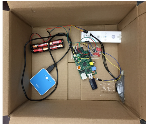
Fig. 3: SHAZam Internal Hardware. Clockwise, from top: Wiimote, Sparkfun RS485 breakout board, Raspberry Pi with attached Bluetooth dongle, USB power module for the Raspberry Pi, Battery assembly (8 AA) for powering motors.
